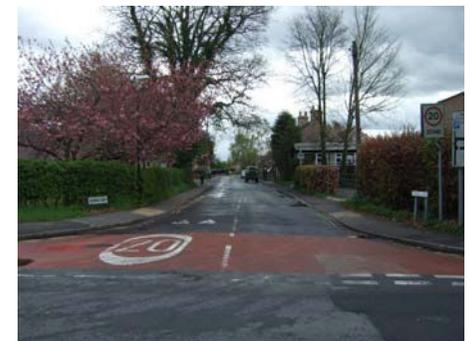
Plate 50 Excessive signage and road markings
